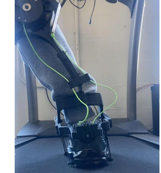
\*Previous iteration of Exoskeleton with beam spring for series elasticity instead of Spring Mechanism
