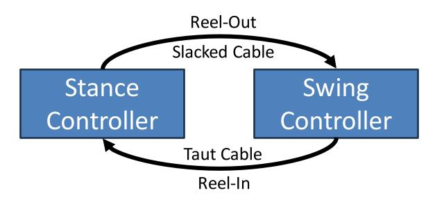
However, to make this transition smooth we need series elasticity with: - Low Stiffness during Swing - High Stiffness during Stance
